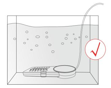
B.Plug to power and gently touch the "SET" button on the IC temperature controller and you will see the digital temperature flashing three times on the display of heater. Press the " — " or " + "button until reach your desired temperature value. The display will flash the desired temperature value three times, then return displaying the current water temperature. Your setting is done. You can press the " — " or " + " button persistently to display 70~94°F in a cycle.
