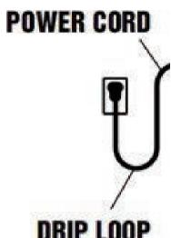
NOT unplug the cord. Disconnect the fuse to the circuit breaker that supplies power to the heater. Then unplug and examine for the presence of water in the receptacle.
